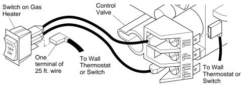
Figure 31 - Connecting Wire Terminals
